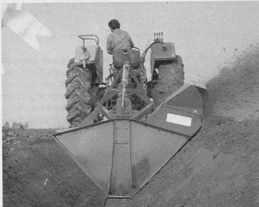
Photo 1 Tractor-drawn rotary-blade ditcher at work. (By courtesy of Impex International, Spartanburg, South Carolina, USA)
