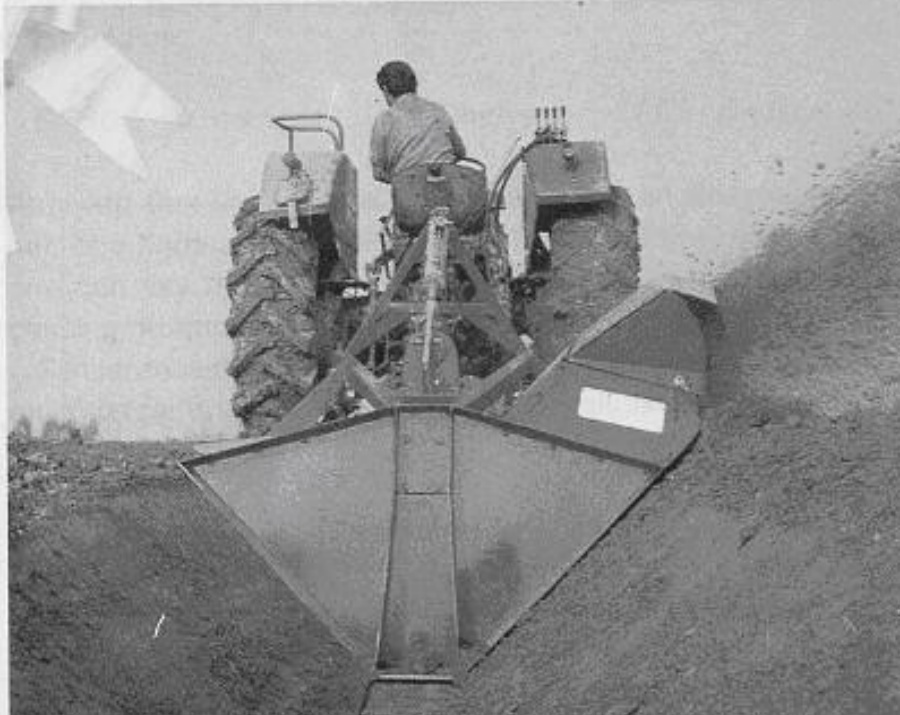
Photo 1 Tractor-drawn rotary-blade ditcher at work. (By courtesy of Impex International, Spartanburg, South Carolina, USA)
