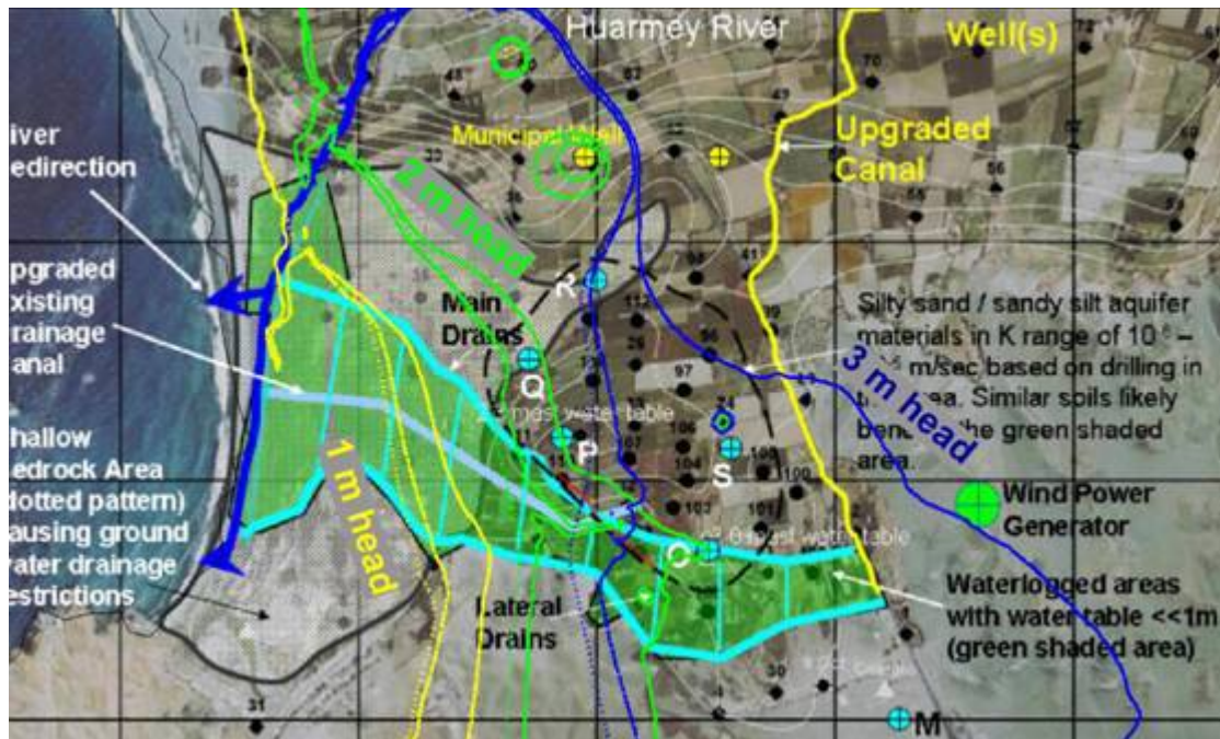
Figure 5. Simulation of groundwater levels after implementing a drainage system using FEFLOW
