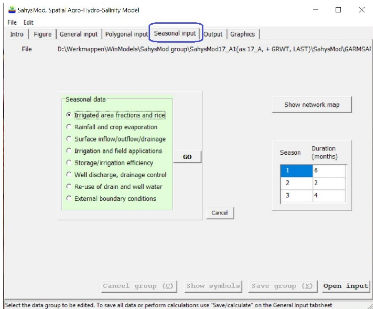
Figure 7. The SahysMod “Seasonal input” tab sheet (blue square) contains the seasonal data for each polygon. It can be seen that in this case the model uses three seasons in a year, as is also evident in figure 3..
