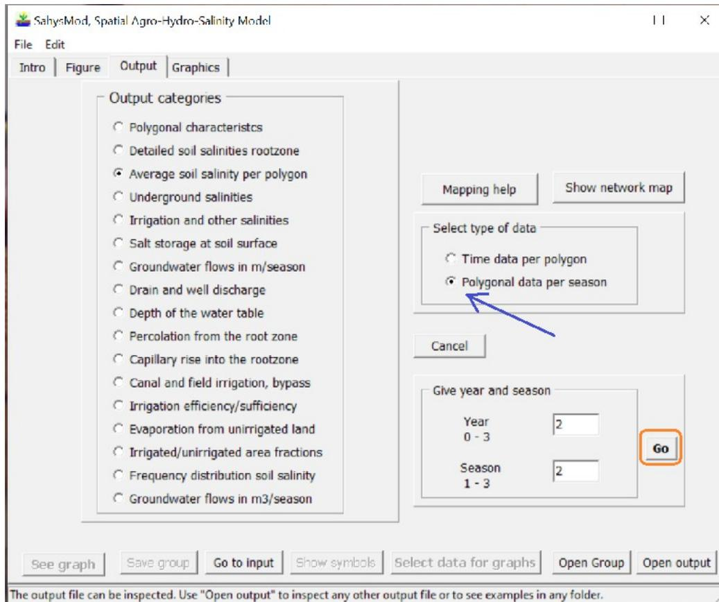
Figure 14. Instead of the choice “Time data per polygon” in figure 11, here the option “Polygonal data per season” is chosen (blue arrow) and the season selected is the second one (of three) in the second year (of three).
