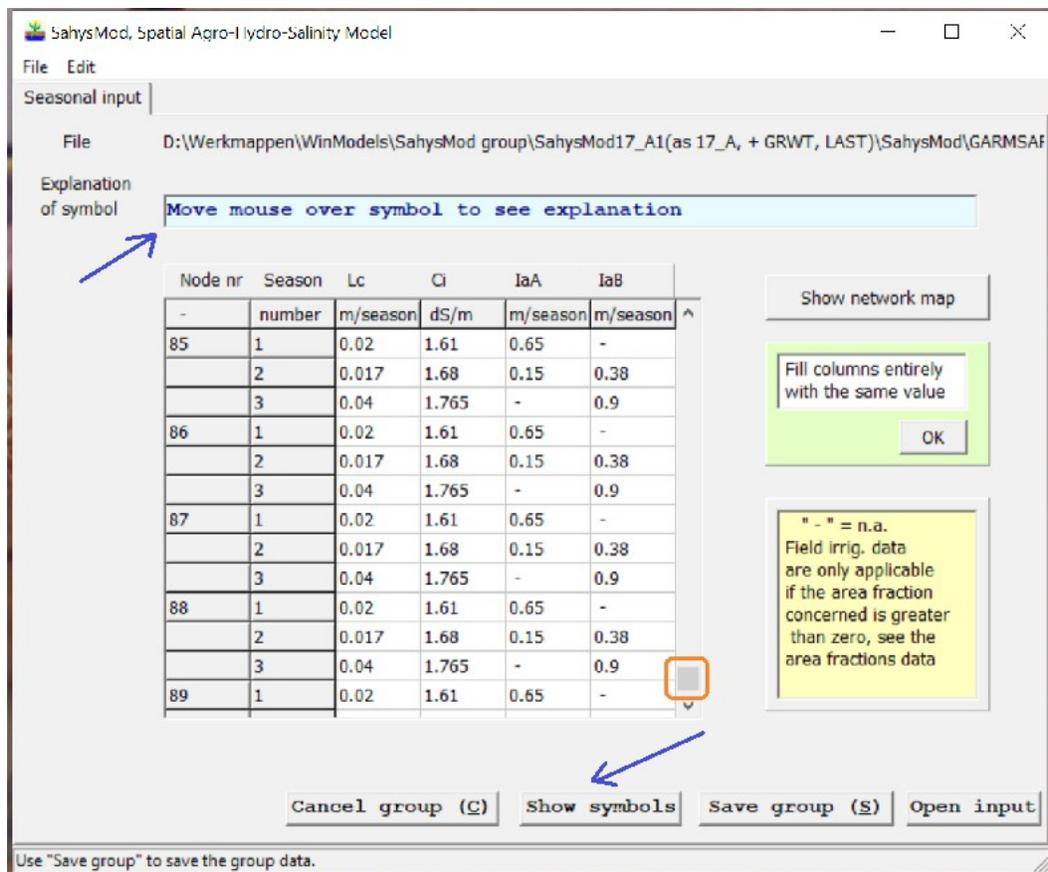
Figure 8. Table of irrigation data. There are two ways to find the meaning of the symbols used (blue arrows). In this picture the seasonal irrigation data are shown for polygons 85 to 88 because the scroll bar (orange square) has been moved down.
