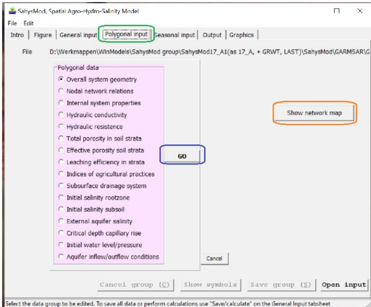
Figure 4. The “Polygonal input” tab sheet (green square) reveals a table (rose colored) with items concerning the data that need to be known for each polygon. The selection in this figure is “overall system geometry” Clicking the “Go” button (blue square) will give the details of the geometry required. The “Show network map” button (orange square) will provide a picture of the polygonal network employed.
