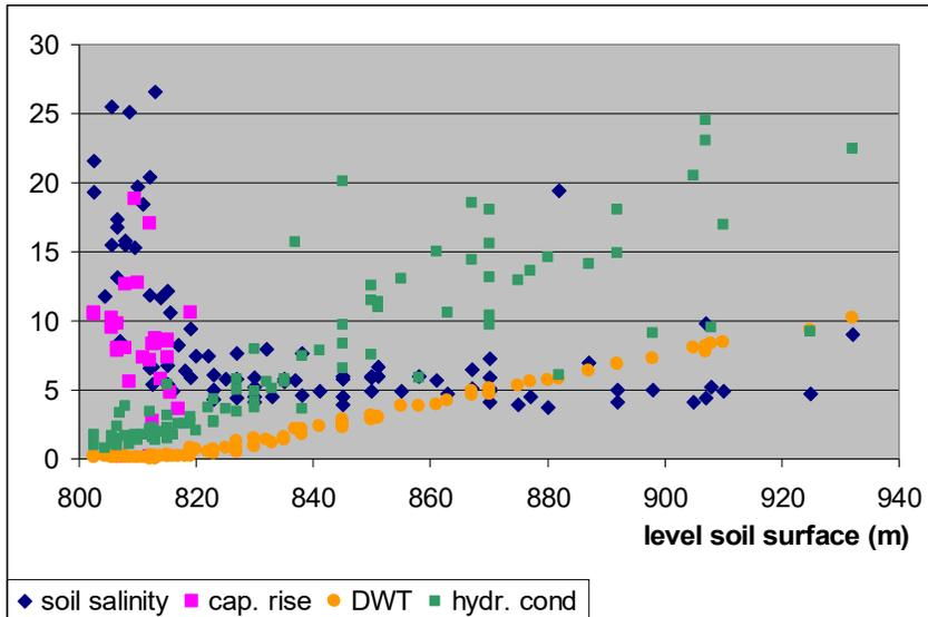
*Legend: soil salinity in dS/m, cap. rise = capillary rise in cm/day, DWT = depth of the water table in units of 10 m, hydr. cond = hydraulic conductivity of the aquifer in units m<sup>3</sup> per day. The units have to be adjusted so that they can be plotted against the same Y-axis.*
