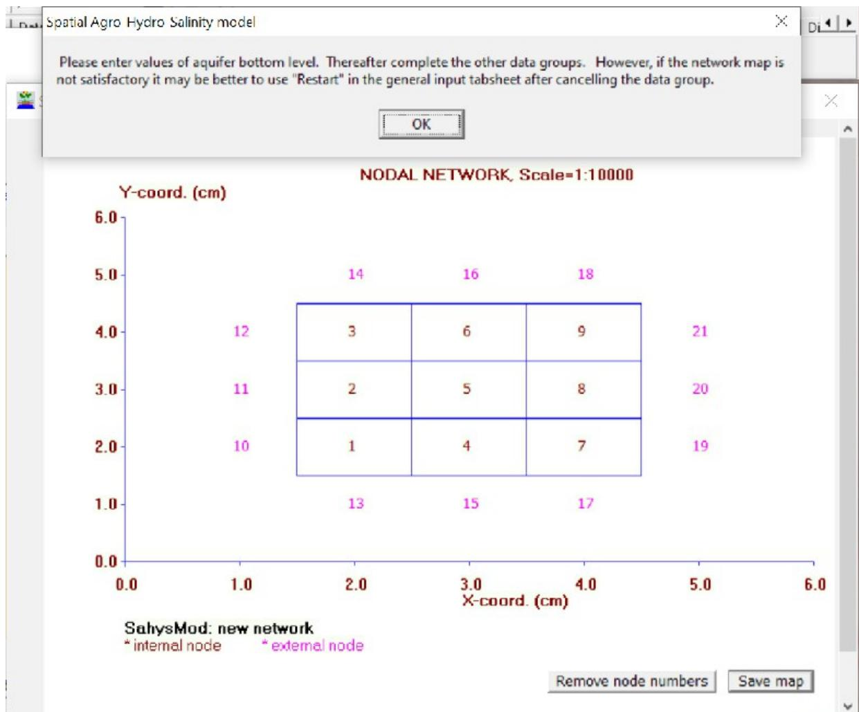
*This picture shows the polygonal network that has been created with the data previously provided.*
