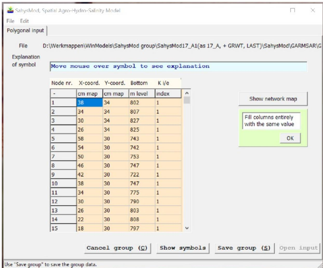
Figure 5. The geometry data filled in for each polygon. There X and Y coordinates, level of the bottom of the aquifer and the K index, which stands for the key of rotational type of agricultural land use,  $K = 0, 1, 2, 3$  or  $4$ . The explanation of the K index can be found clicking on the “Show symbols” button.
