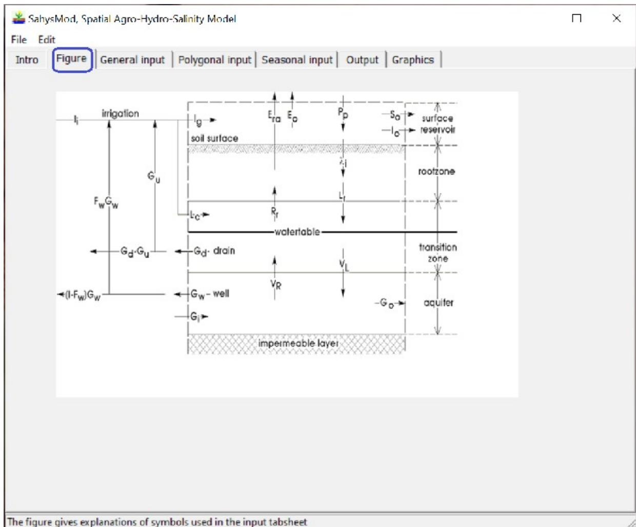
Figure 2. The “Figure” tab sheet is opened (blue square). It gives a schematic overview of the physical elements used in the polygons of SahysMod. It shows the hydrology, the irrigation canal system, ground water use, and three soil layers as used in each of the polygons, though specific characteristics may differ between the polygons.
