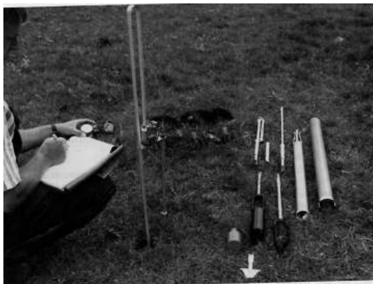
Figure 12.14 Equipment used for the auger-hole method (van Beers 1970)
