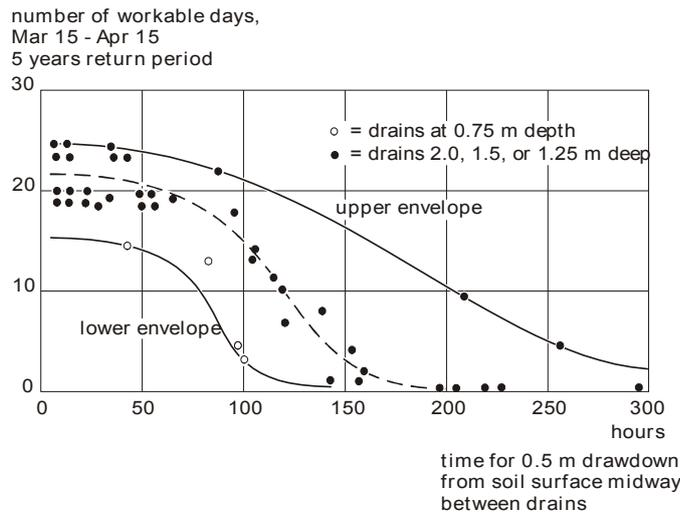
Figure 17.11 A plot of draw down time of the water table versus number of workable days for different drainage systems in North Carolina, U.S.A. (Skaggs 1980)
