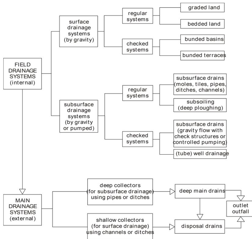
Figure 17.1 Classification of types of agricultural drainage systems
